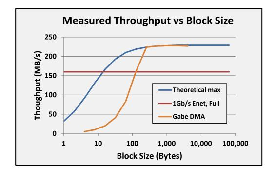
Note 1: Theoretical Max bounded by context switching Note 2: Un-optimized generic Altera DMA Interface Note 3: CUDA style DMA planed for next generation
